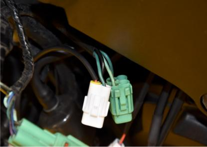
Release the Green/Red and Black/Blue male terminals out from the larger side of the gear position sensor connector.
