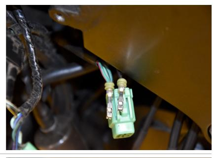
Insert the two female terminals to the smaller 3-pole plug adapter.
